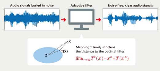
Fig. 1 Adaptive filter: its application example and basic principle
