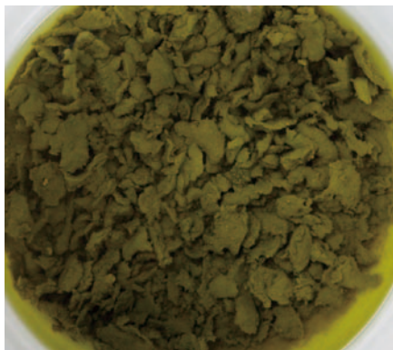
(Left) Marine cyanobacteria are being extracted using an organic solvent. After several days of extraction, the liquid is filtered and enriched in an extract. / (Right) For research involving chemical synthesis, thin layer chromatography (TLC) is employed to examine the progress of reactions. TLC can also be used as a means for separation.
