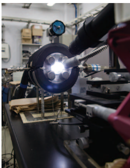
Using this equipment which looks like a cylinder placed in a horizontal position, we can observe the crystal growth process of clathrate hydrates under high pressures and low temperatures. The image above shows a hydrate crystal that is growing through a reaction between methane + CO 2 mixture gas with water.
